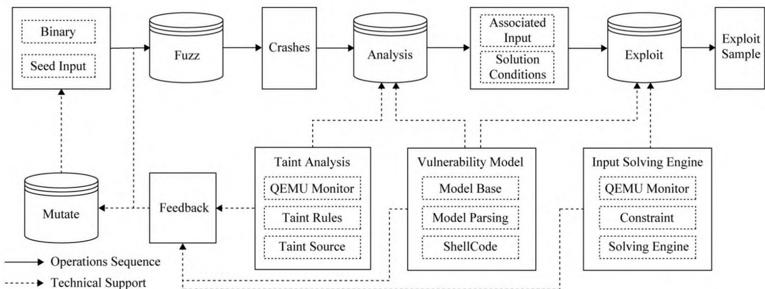
Fig.7 Framework of prototype system
