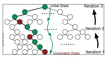
Figure 3. Backward symbolic execution strategy: we search for a path from the last cycle to the first cycle (black arrows). Within each cycle, we symbolically execute the hardware design forwardly (green arrows).
