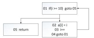
FIGURE 8. The loop statement in Code 3 to the control-flow of the conditional branch statement.
