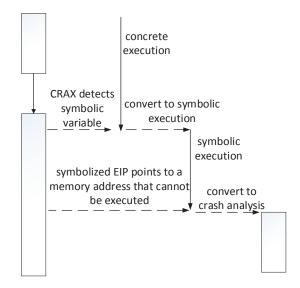
FIGURE 4. The process of the transformation from symbolic execution to crash analysis.
