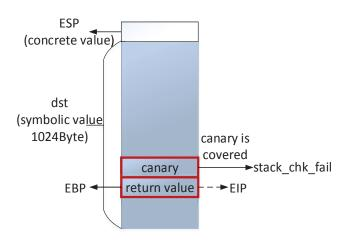
FIGURE 5. The stack frame of Code 1 under the protection of canary.
