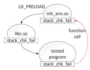
FIGURE 9. The API is hooked in init\_env.so through LD\_PRELOAD.
