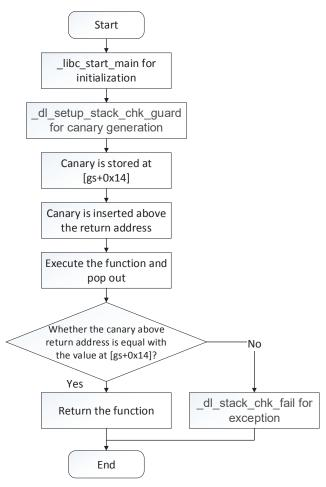
FIGURE 3. The canary mechanism workflow in 32-bit Linux.
