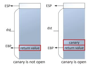
FIGURE 2. The two states of the canary in stack frame.
